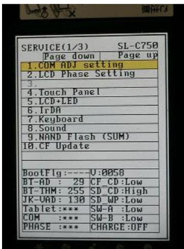
Navigation within the menu is possible with the stylus, the arrow keys or the scroll wheel.
